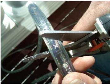
Using a good set of cutting shears, you can cut IlluminFx LED rope light wherever the "X" is (this is actually a scissors symbol). Cutting anywhere else will damage the rope light.
