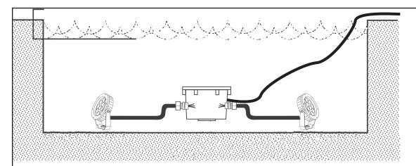
Connect you main power or data line up to the SS-JB. (EX: If using the SS-JB4, wire 3 lighting fixtures into the Junction box). Connect each wire with a wire nut, making sure to maintain the correct polarity. Tighten down each compression fitting to ensure a good seal. It is recommended to then test on dry ground to make sure all the lighting fixtures are working correctly.
