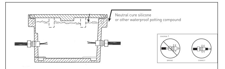
Make sure you have fed the wires all the way into the compression fitting (diagram 1). It is recommended to then fill the cavity of the SS-JB with a neutral cure silicone of potting compound to ensure complete IP68 protection. Finally, place the lid on the junction box and tighten down with the (6) Stainless steel bolts provided with each junction box.
