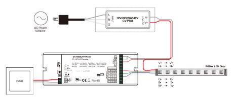
Note: please make sure the dial switches are at position for RGBW mode as shown in above diagram.
